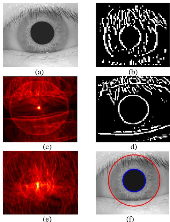
Figure 13. (a) Original eye image (CASIA: 47\_1\_1.bmp) from CASIA database, (b) Vertical edge of eye, (c) Hough transform, (d) Horizontal edge map, (e) Hough transform image showing center of the iris, (f) Localized iris image. Figure.14. shows simple implementation of the iris unwrapping.
